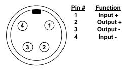
Figure 1 – AMP-15 Female Connector Pin Out
